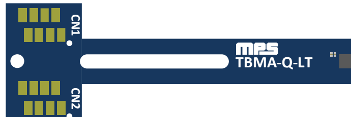
Figure 1: TBMA Test Boards
