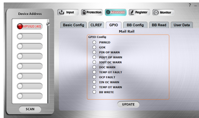
Figure 7: GUI Advanced Page, GPIO Tab
