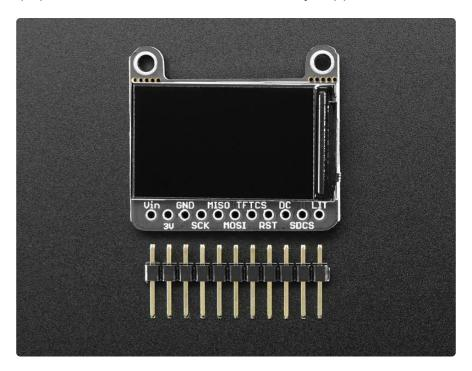
Our breakout has the TFT display soldered on (it uses a delicate flex-circuit connector) as well as a ultra-low-dropout 3.3V regulator and a 3/5V level shifter so you can use it with 3.3V or 5V power and logic. We also had a little space so we
