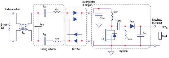
Figure 2: Schematic diagram of the EPC9514 demo board.
