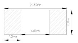
Recommended trace thickness is 35 um; the minimum trace width is 5 mm Recommended stencil thickness is 0.15 mm
