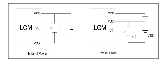
$V_{DD^{\sim}}V_0$ : LCD Driving voltage
