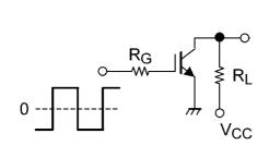
Fig. 6.2.1 Test Circuit of Switching Time
