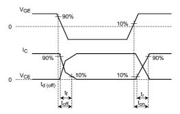
Fig. 6.2.2 Timing Chart of Switching Time
