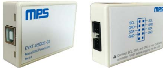
Figure 3: USB to I 2 C Communication Kit
