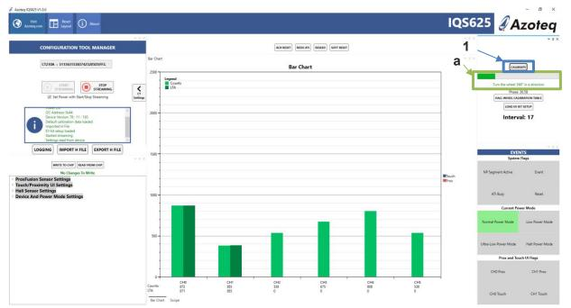
Step 2: Complete one full rotation until the "Calibration Completed" message is received. (Repeat step 1 if the message: "Calibration Failed" is received.)
