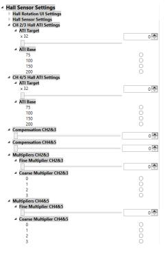
The ATI process adjusts three values (Coarse multiplier, Fine multiplier, Compensation) using two parameters per plate (ATI base and ATI target). The ATI process is used to ensure that the sensor's sensitivity is not severely affected by external influences (Temperature, voltage supply change, etc.).
