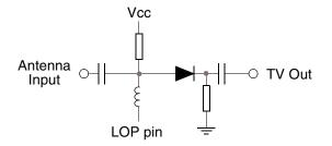
Figure 6. Attenuator Application with PIN Diode
