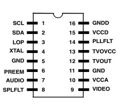
Figure 1. MC44BC373C/4C Pin Connections
