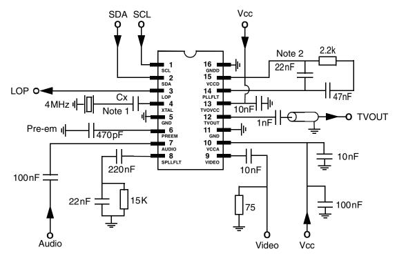
Note 1: Cx value depends on crystal characteristics; Cx = 27 pF on Motorola application board. Note 2: Loop Filter components must be as close as possible to pins 14 and 15.
