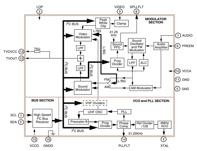
Figure 2. MC44BC373C/4C Simplified Block Diagram
