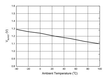
Shutdown Voltage vs. Ambient Temperature
