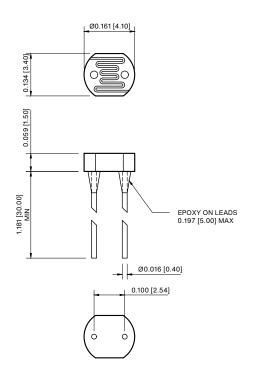
Note: Lead soldering temperature (1/16 inches away from body) 260°C for 3 sec.
