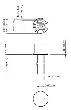
Note: Lead soldering temperature (1/16 inches away from body) 260°C for 3 sec.
