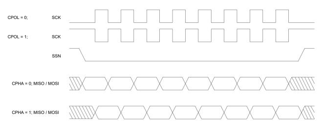
**NOTE:** In the BCM53154/BCM53156/BCM53158, the maximum SPI slave SCK frequency can be 25 MHz when the internal clock is 400 MHz and 20 MHz when internal the clock is 200 MHz.
