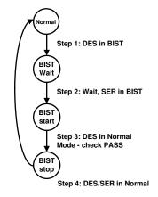
Figure 28. BIST Mode Flow Diagram
