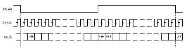
Figure 22. I2S Frame Timing Diagram
