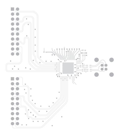
Figure 44. DS90UB947N-Q1 Serializer Layout Example
