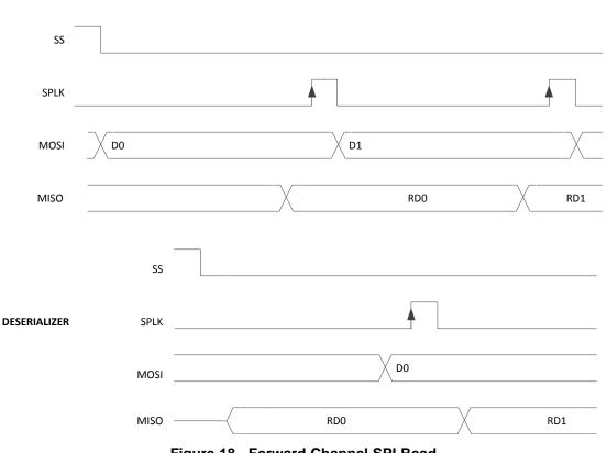
Figure 18. Forward Channel SPI Read
