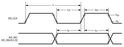
Figure 9. I2S Timing Diagram
