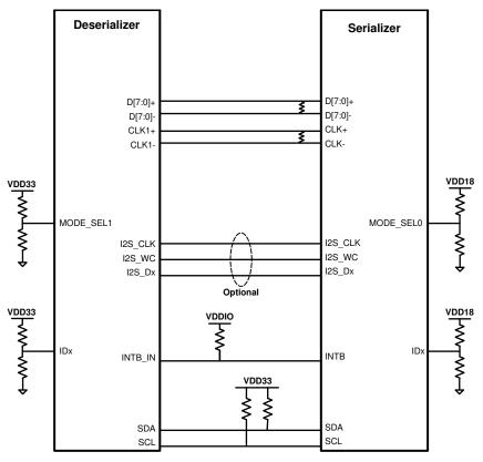
Figure 26. Repeater Connection Diagram
