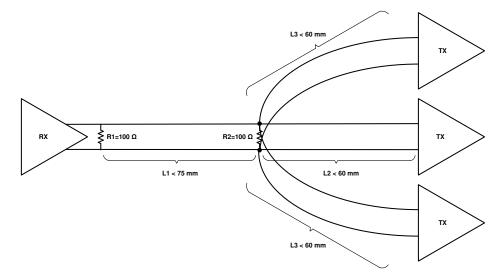
Figure 27. FPD-Link Fan-Out Electrical Requirements
