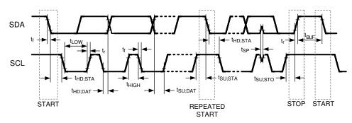
Figure 8. Serial Control Bus Timing Diagram
