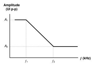
Figure 31. Input Jitter Tolerance Plot
