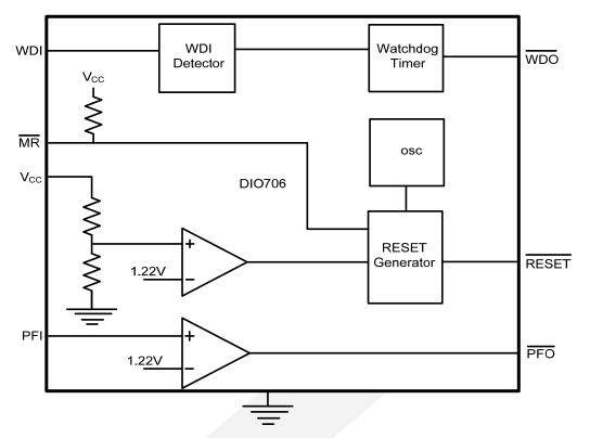
Figure 2 DIO706 Block Diagram
