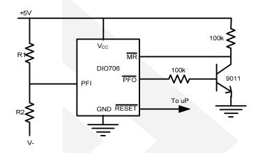
Figure 7 Monitoring A Negative Voltage
