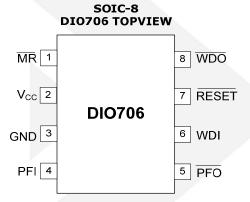
Figure 1 Pin Assignment
