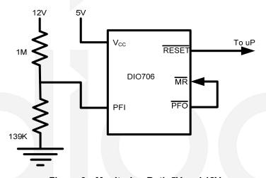
Figure 6 Monitoring Both 5V and 12V
