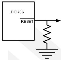
Figure 5 RESET Valid to Ground Circuit
