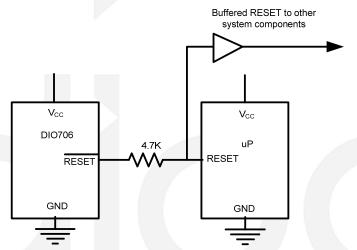
Figure 8 Interfacing to uPs with Bidirectional Reset I/O
