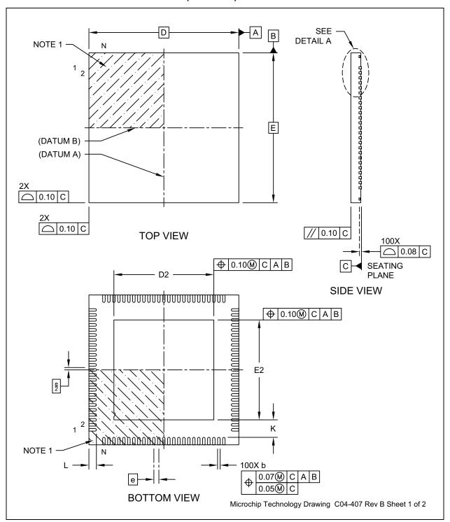
FIGURE 10-2: 100-VQFN PACKAGE (DIMENSIONS)
