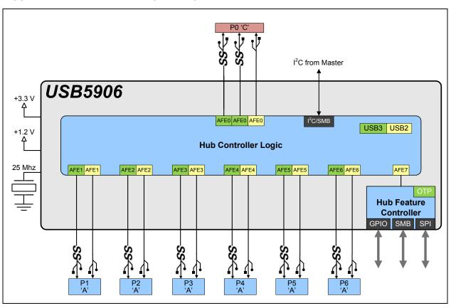
FIGURE 2-1: INTERNAL BLOCK DIAGRAM
