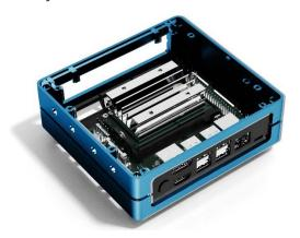
**Stackable structure to extend endless possibilities for building different applications such as NAS.** If your application requires more space, for example, adding more hard disks to make a NAS, the stackable structure allows you to stack more middle layers to create rooms very easily.
