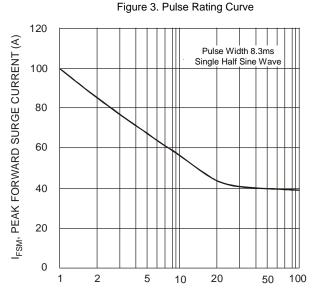
NUMBER OF CYCLES AT 60Hz Figure 5. Maximum Non-Repetitive Surge Current
