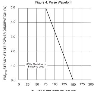
$\label{eq:TL} {\rm T_L,\, LEAD\,\, TEMPERATURE\,\, (^{\circ}{\rm C})}$  Figure 6. Steady-State Power Derating Curve
