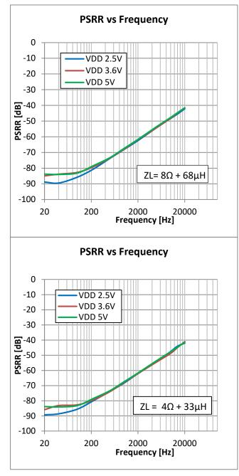
Note : The above PSRR plots are captured with input capacitors 2.2uF
