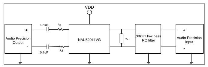
Note: The 30kHz low pass RC filter is implemented by using R= 1k Ohm and C = 4.7nF
