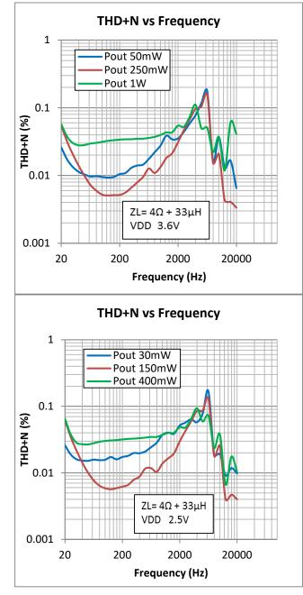
Note: All the above plots are captured with 0.1uF input capacitor. It is recommended to use 2.2uF input capacitor to get a flat low frequency response.
