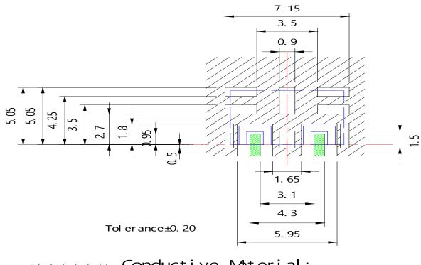
Conductive Material: Ground, connected to lower ground diameter of 0.3mm and max. distance of 1.0mm
