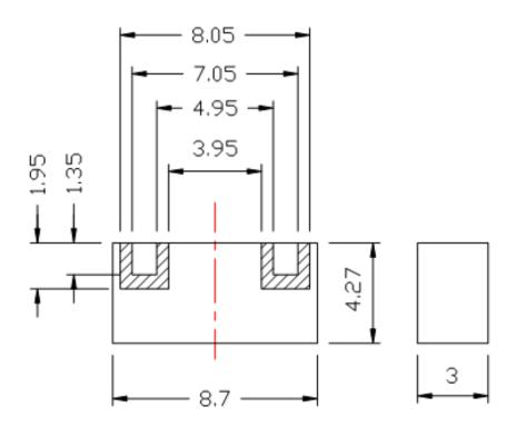
Dimensions in mm Tolerance : ±0.25
