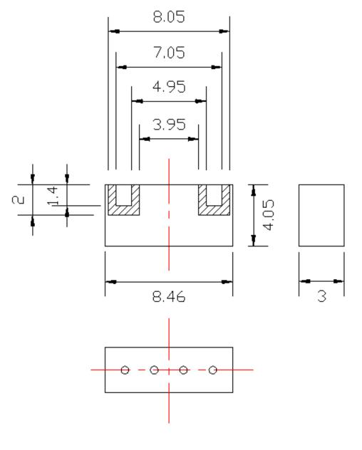
Dimensions in mm Tolerance:±0.25
