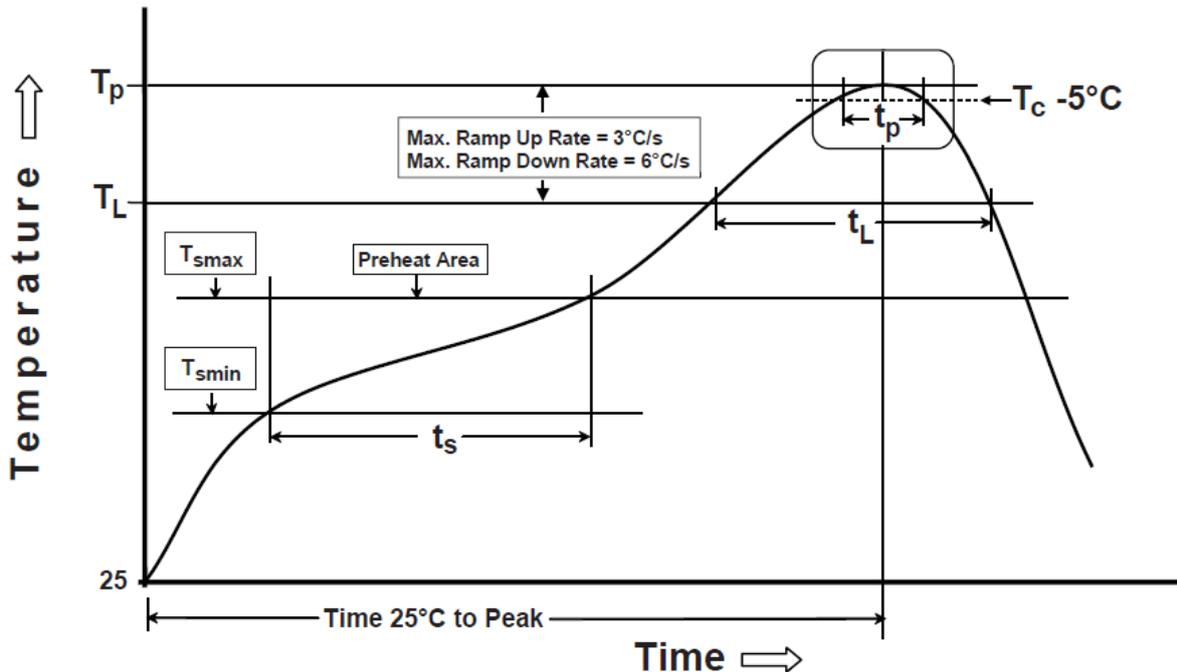
Table Pb-free Process – Package Peak Reflow Temperatures
