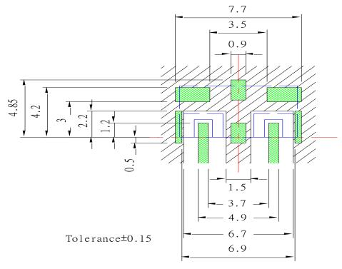
Conductive Material: Ground, connected to lower ground diameter of 0.3mm and max.distance of 1.0mm.
