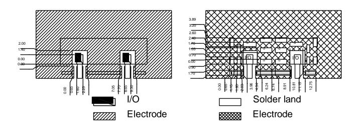
The recommended shielding case layout guide (min)
