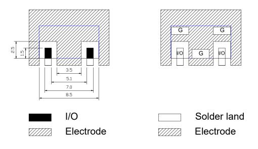
Shielding case layout guide (MIN)
