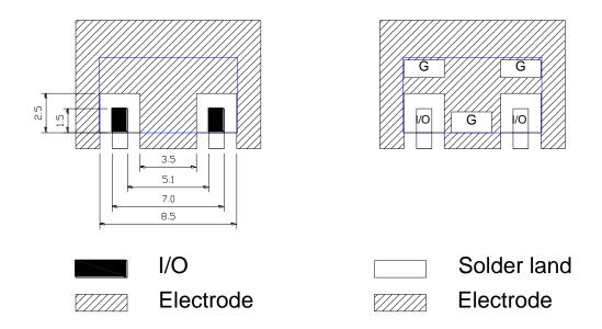
Shielding case layout guide (MIN)
