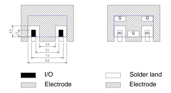
Shielding case layout guide (MIN)
