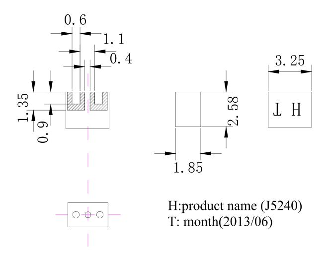
Dimensions in mm Tolerance:+/-0.2
