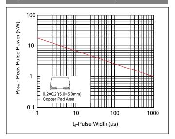
Figure 2. Pulse Derating Curve
