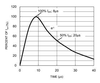
Fig.7 ESD pulse waveform
