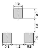
Fig. 4-3: SOT23 footprint for reflow soldering
