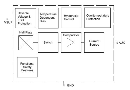
Fig. 3–1: HAL 156y block diagram
