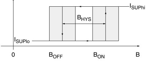
Fig. 4-11: Definition of magnetic switching points for the HAL 1566
