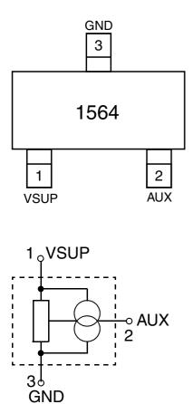
Fig. 4–5: Pin configuration
