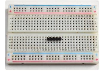
Prepare the header strip: Cut the strip to length if necessary. It will be easier to solder if you insert it into a breadboard - long pins down.
