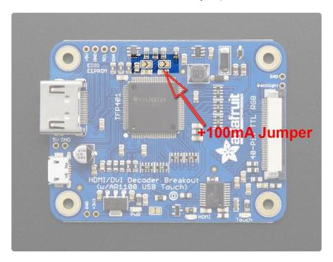
If you are using a 7.0" diagonal screen, chances are its a 125mA backlight - the ones we sell in the Adafruit shop are 125mA. If not using an Adafruit screen please check, as we have also seen some backlights that are 50mA! You can run it at 25mA but it will be very dim. You should close the +100mA jumper
