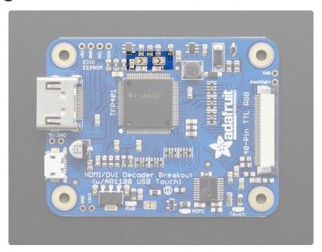
This is a generic TTL display driver, and each display has a slightly different backlight configuration. For that reason, you may need to make some adjustments to your board.
