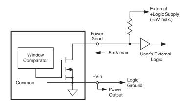
HI impedance (Open Drain) = Power Ok LO impedance (Saturation) = Power Not Ok
