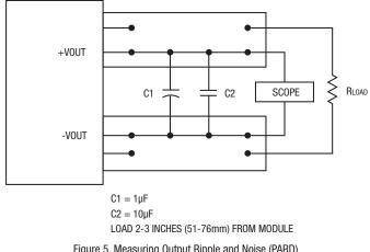
Figure 5. Measuring Output Ripple and Noise (PARD)
