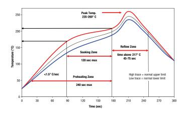
Recommended Lead-free Solder Reflow Profile
