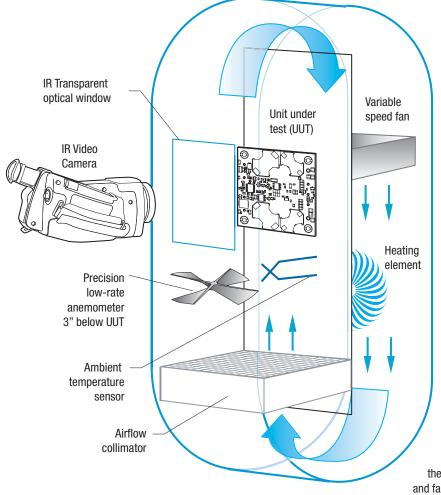
Figure 9. Vertical Wind Tunnel
