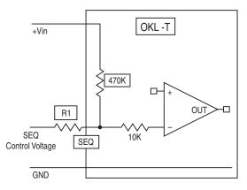
Figure 7. Sequencing Signal Interface of Module
