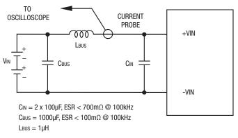
Figure 4. Measuring Input Ripple Current
