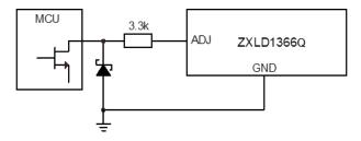
If the NMOS transistor within the microcontroller has high Gate / Drain capacitance, this arrangement can inject a negative spike into the ADJ input of the ZXLD1366Q and cause erratic operation, but the addition of a Schottky clamp diode (eg Diodes Incorporated SD103CWS) to ground and inclusion of a series resistor (3.3k) will prevent this. See the section on PWM dimming for more details of the various modes of control using high frequency and low frequency PWM signals.
