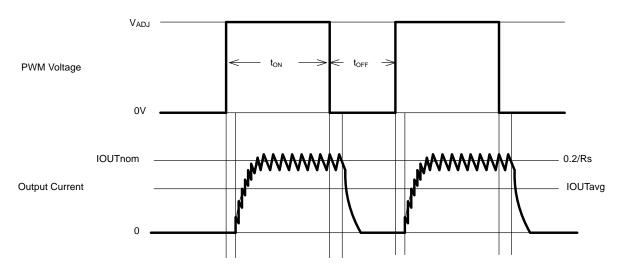
Figure 8. Low Frequency PWM Operating Waveforms
