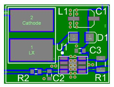
Figure 7. Suggested Layout for SO-8EP Package
