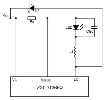
Figure 6. Reduced Output Ripple
