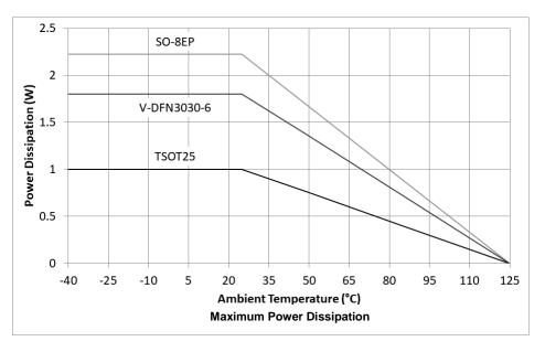
Note that the device power dissipation will most often be a maximum at minimum supply voltage. It will also increase if the efficiency of the circuit is low. This may result from the use of unsuitable coils, or excessive parasitic output capacitance on the switch output.
