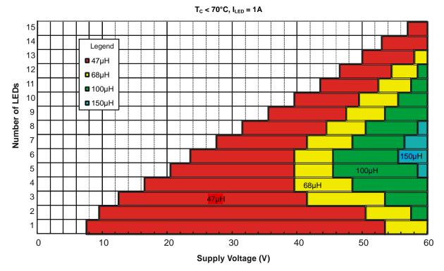
Figure 4. ZXLD1366Q Minimum Recommended Inductor (SO-8EP)
