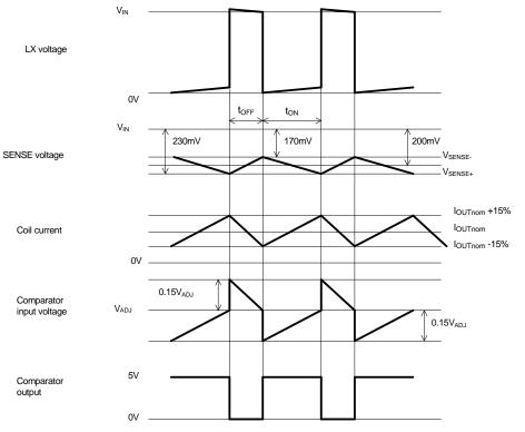
Figure 2. Theoretical Operating Waveforms
