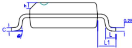
Figure 4. 8-Lead Small Outline Package [SOP]
