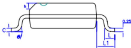
Figure 4. 8-Lead Small Outline Package [SOP]
