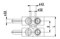
The plug-in terminal strip 302-STS is available in 8 mm pitch with 1 to 12 poles. It has one screw connection per pole and one vertical pin for the connection to the socket of the female counterpart.
