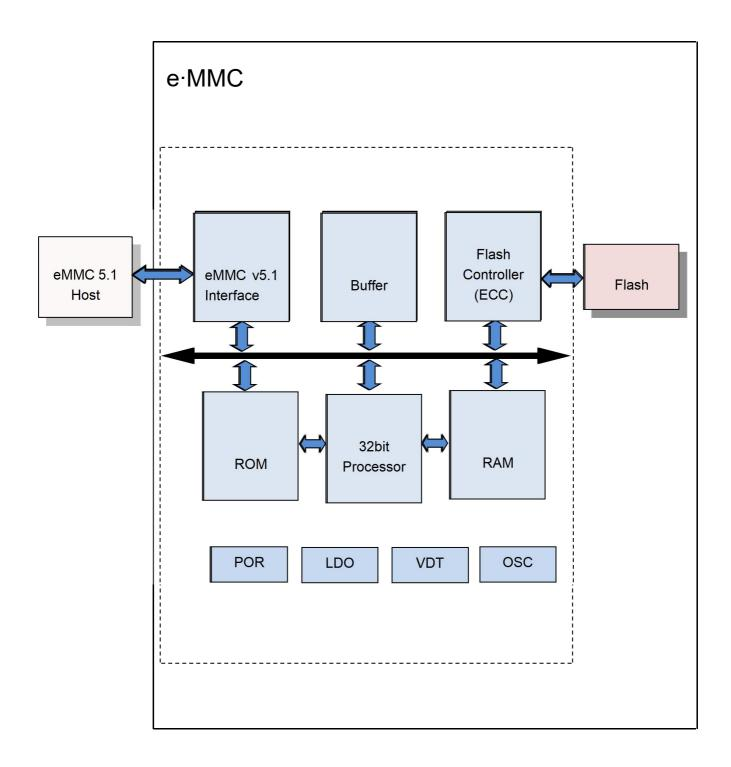
Figure 1 - e·MMC Block Diagram
