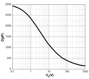
Fig. 5 - Capacitive Charge vs Reverse Voltage
