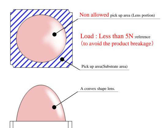
Please adjust the load, the pick up point, the nozzle diameter and etc. before mounting because the over load can cause the breakage of the surrounding of LED.
