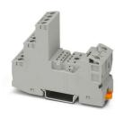
RIF-2... relay base, for industrial relay with 2 or 4 changeover contacts, screw connection, plugin option for input/interference suppression modules, for mounting on NS 35/7,5
