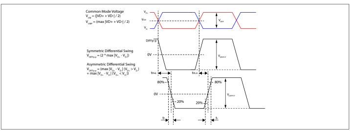
Figure 4. Definition of Peak-to-peak Differential Voltage
