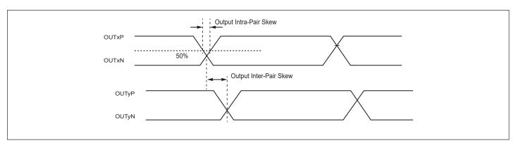
Figure 10. Intra and Inter-pair Differential Skew Definition
