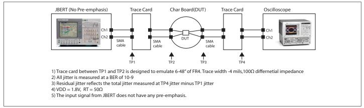
Figure 8 Channel Measurement Setup
