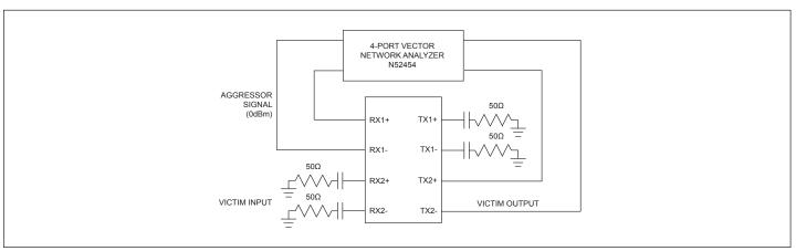
Figure 7. NEXT Channel-isolation Test Configuration
