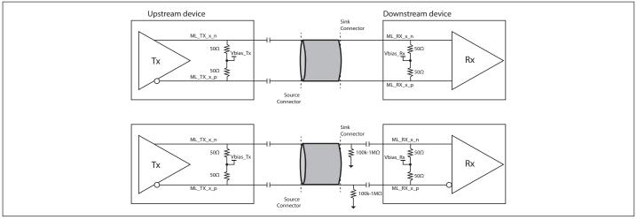
Figure 9. High-speed Channel Test Circuit
