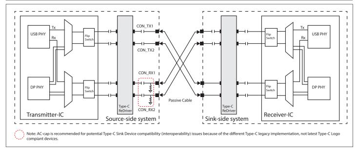
Figure 13. Type-C Coupling Capacitor Connection Diagram
