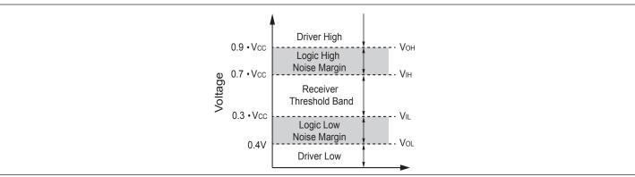
Figure 11. I2C I/O Stage Noise Margin
