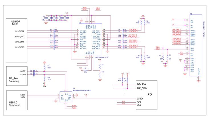
Figure 14. Type-C DFP Application Schematic
