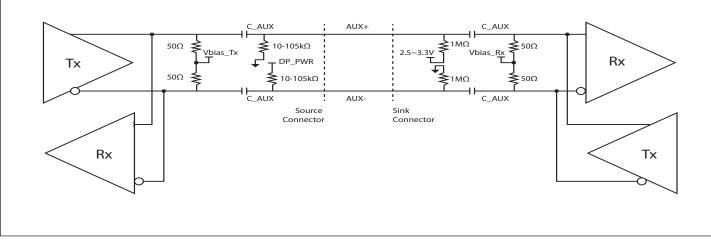
Figure 3. DisplayPort AUX Channel Connection
