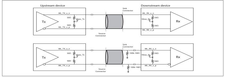
Figure 1. DisplayPort Main Link Connection Diagram
