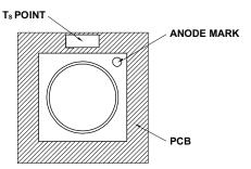
$T_S$  can be easily measured by mounting a thermocouple on the soldering joint as shown in preceding figure, while  $R_{\theta J\text{-}S}$  is provided in the data sheet. Verify the  $T_S$  of the LED in the final product to ensure that the LEDs are operating within all maximum ratings stated in the data sheet.
