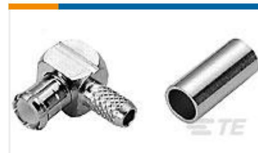
TE Part #1-1337585-0 MCX R/A Plg Hex 50Ohm Gold Pltd RG174A/U
