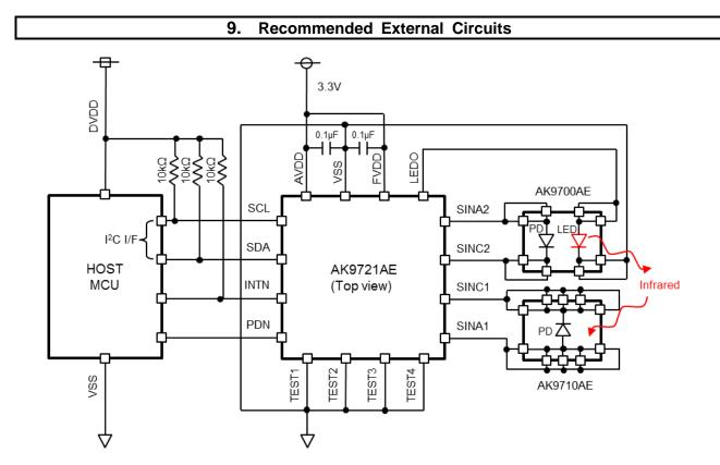
Figure 9.1 Recommended External Circuits
