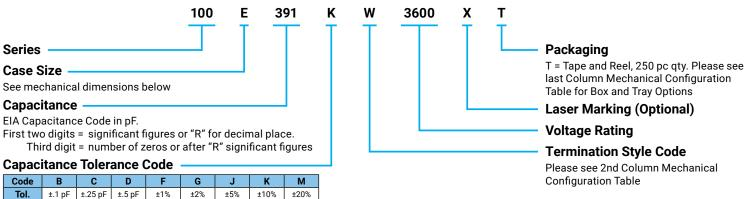
The above part number refers to a 100 E Series (case size E) 390 pF capacitor, K tolerance (±10%), 3600 WVDC, with W termination (Tin / Lead, Solder Plated over Nickel Barrier), laser marking and Tape and Reel packaging.
