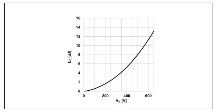
Figure 5 Typical capacitance stored energy;  $E_c = f(V_R)$
