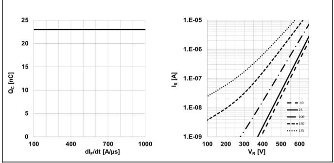
Figure 3(LEFT) Typical capacitive charge versus current slope (only capacitive charge, guaranteed<br/>by design);  $Q_c = f(di_F/dt)$ ;  $T_j = 150^{\circ}C$ ;  $V_R = 400V$ ;  $I_F \le I_{F,max}$ <br/>(RIGHT) Typical reverse current versus reverse voltage;  $I_R = f(V_R)$ ; parameter:  $T_i$
